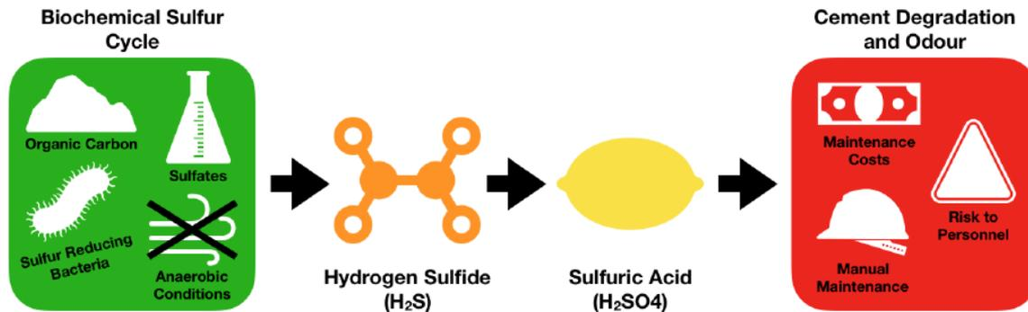
Above - Schematic of sewage odour and corrosion generation Image
